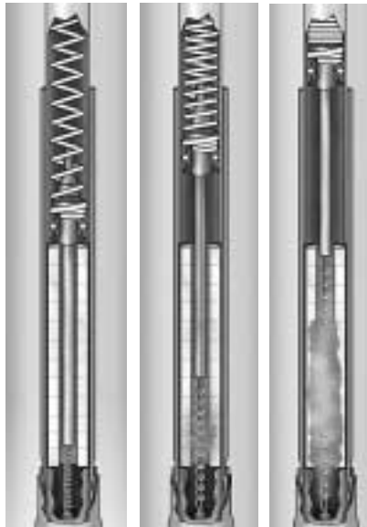
Element Melts Rod withdraws, elongating arc and vaporizing Boric Acid Vapor quenches arc at first current zero
