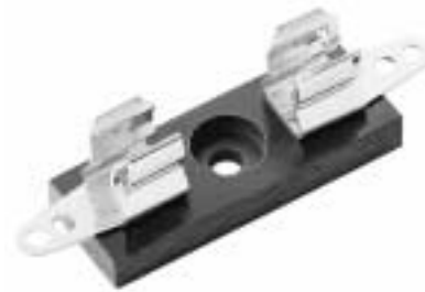
4520 and 4393 Single Pole Fuseblock for 1/4" x 1" Fuses Bakelite base; Width 1/2" (12.7mm). Spring-bronze, bright tin-lead plated clips. Rated 30A, 250V.
